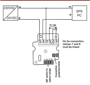
The output voltage is temperaturelinear. It should be noted that output is only controllable up to ca. 0.02V, relative to the below supply voltage.
