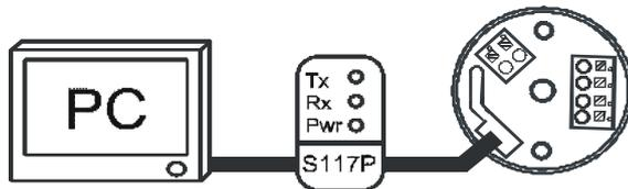
The mating connector of the measurement transducer is hidden under a plastic covering cap. Lift and turn this cap as depicted in the illustration. The transmitter is powered via the programming cable.
