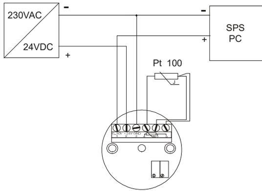
The output voltage follows the temperature signal at input linearly. It must be noted that the output only allows control to within approx. 0.02 V at the lower supply voltage.
