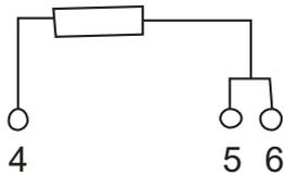
The Type 424 can also be operated as a **two lead circuit** by short circuiting across clamps 5 and 6. In this case the resistance of the leads does affect the results measured. The null point potentiometer can be adjusted to make small corrections. The range potentiometer should be adjusted as little as possible.
