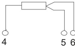
The Type 424 measurement converter is operated as a **three lead circuit**, i.e. the resistance of the leads does not affect the results measured, if the leads are of equal length and made of the same material.
